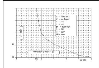
Effect of pressure p<sub>2</sub> on noise pressure level generated by a 14" x 28" Limiphon discharging to condenser
