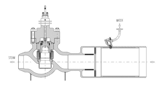
1-9154 - Limiphon reducing/desuperheating valve straight-way cast body - bottom inlet- filtering basket under the seat - balanced plug with inserts - V leakage class - HAS silencer on the outlet downstream chamber with springnozzle LVL single type - Suitable for moderate flow rates , turn-down and p1/p2 ratios - high pressure differentials - very low noise level
