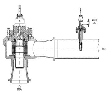
1-9416 Limiphon valve angle body with bottom inlet - sliding and adjustable body/bonnet gasket - balanced plug - filter under seat - V leakage class - downstream chamber with Spraysat desuperheater - Universal solution with no limitation with regard to capacity, turndown, noise control and pressure ratios and differentials
