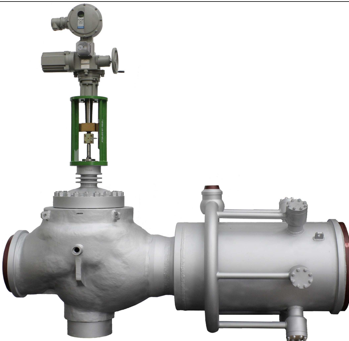
PRDS 1-5945 : 1-6948 DN 20" ANSI 600 with LVM 3-4122 desuperheater installed downstream.
